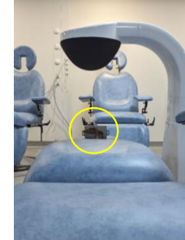
Picture 2: TLA above the seat. Particle counter and fiberglass filter in the breathing zone (yellow circle).
